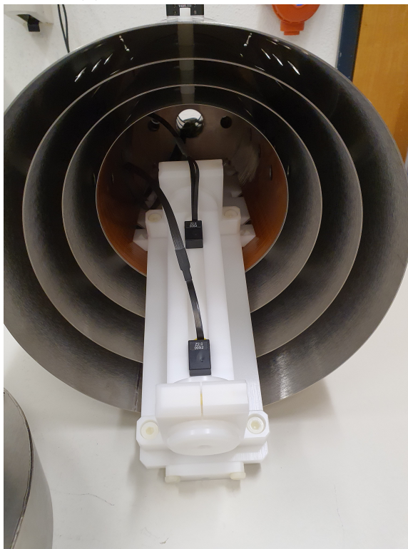
(c) Fixation of the Rb sensors in the holder
