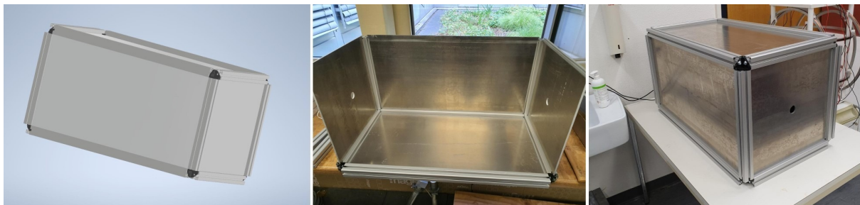
Figure 2.15: Process from sketch to the finished RF shield: The left picture is showing the sketch of the RF shield before ordering the materials. The center picture is showing the assembly of the shield with Item profiles and aluminium plates. The picture on the right shows the finished RF shield containing the Twinleaf mu metal shielding and the Rb-OPMs.
