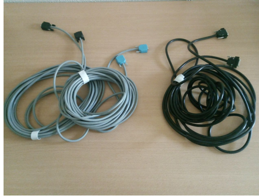
Figure 2.14: Picture of the cables realized to connect the motor and the circuits to the motor control box.
