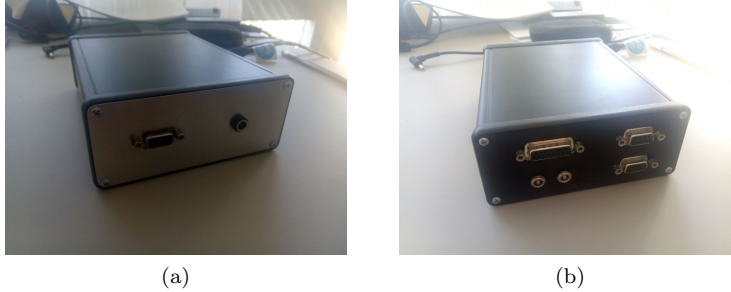
Figure 2.6: Pictures of the motor control box. In (a), the plug for the power supply and the RS-232 plug for the PC-Arduino connection are shown. Figure (b) shows the two D-sub 9 pins connectors for the photodiodes and lasers, the Sub-d 15 pins connector to control the motor and two LEMO plugs to readout the pulse from the photodiode in the open position.
